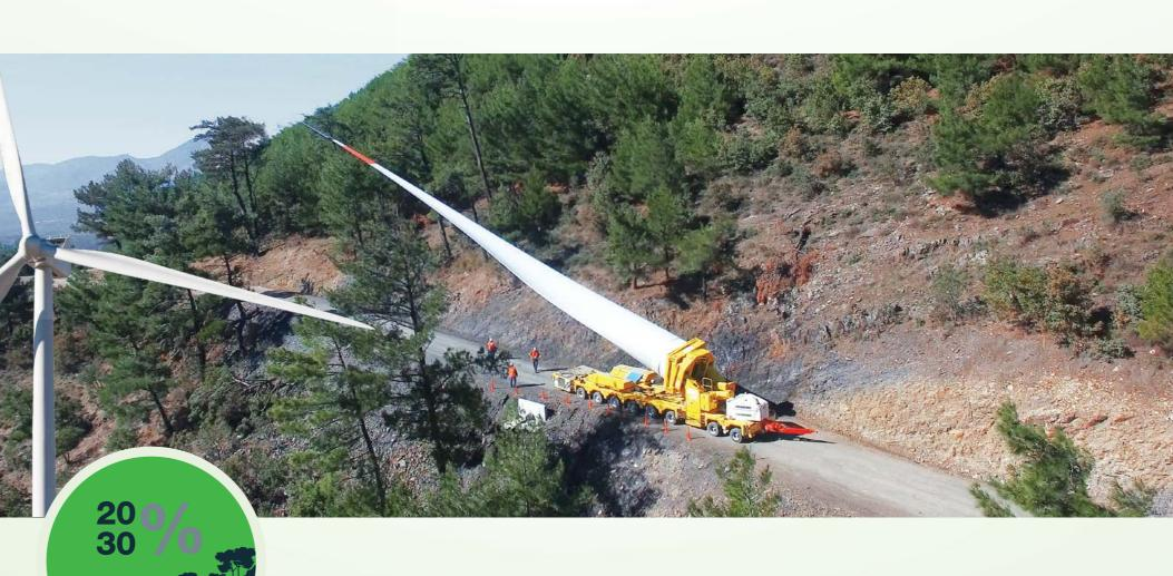
Transportation with the Rotor Blade Adaptor cuts down earthmoving work in rough terrains, slashing negative impact by 20 to 30%.
